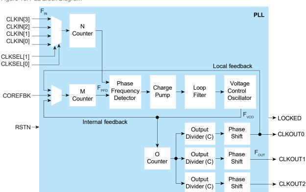
Figure 10: PLL Block Diagram
