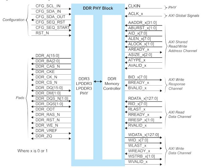
Figure 25: DDR Interface Block Diagram
