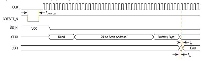
Figure 28: SPI Passive Mode (x1) Timing Sequence
