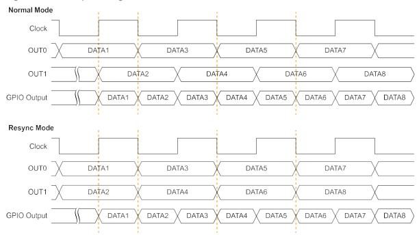
Figure 9: DDIO Output Timing Waveform
