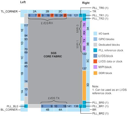
Figure 32: Floorplan Diagram for FPGAs in BGA324 and BGA400 Packages (with DDR and MIPI)
