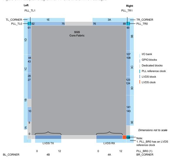
Figure 31: Floorplan Diagram for FPGAs in BGA176 Packages
